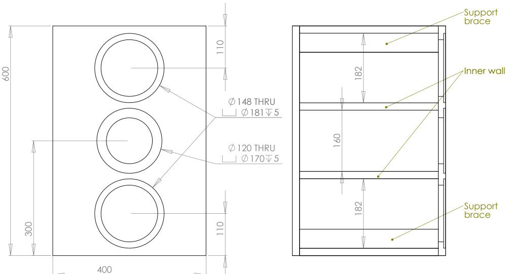
Note: There are two support braces at the top & bottom which are placed 80 mm from the sides, running from rear to front. These are to strengthen the box to support the weight, being between the two woofer boxes.
